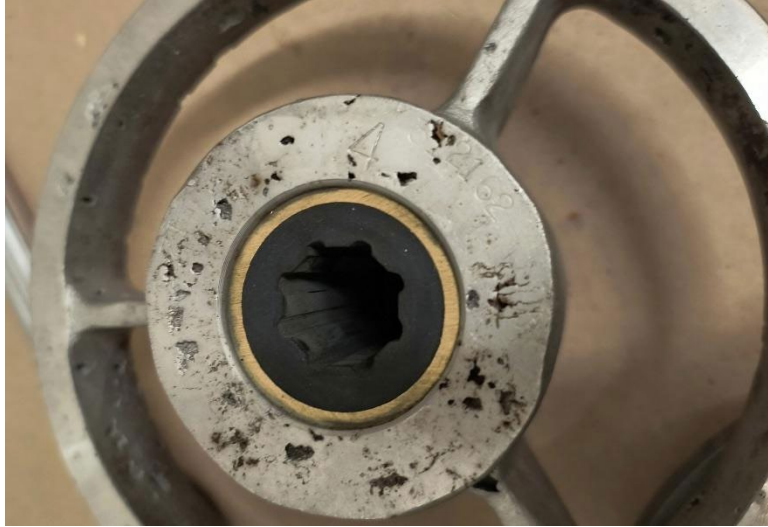
Image 3. LSS-3 line shaft bearings replaced, but with notable pitting and corrosion on metal.
