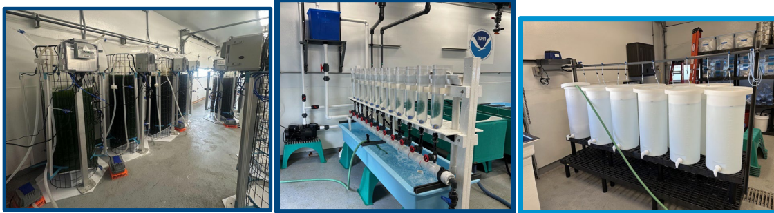
Figure 21. From left: Pure Biomass photobioreactors, bottle upweller system for spat cultivation, larval rearing tanks.
