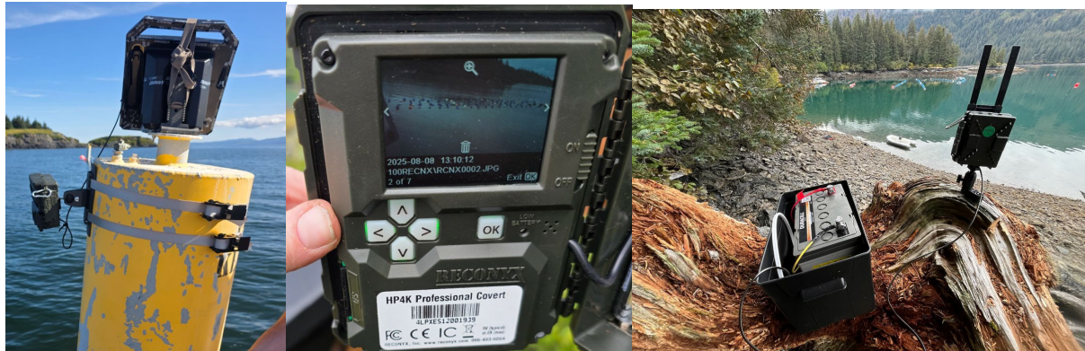
Figure 16. In-use image of Reconyx, Inc. 4k UHD camera (left photo, facing left) and combination solar cell - 105 mAh gel cell battery (top of buoy) installed on an existing buoy at a farm. Cameras are programmed by SD card and sighted on the farm in the field (center photo). Cameras in Jakolof Bay (right) require a larger 50 Ah deep cycle battery due to lack of sunlight.
