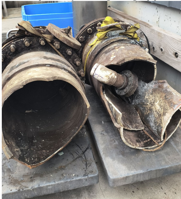
Image. Broken 24" PVC pieces that resulted in the functional loss of one intake line, ready for disposal.
