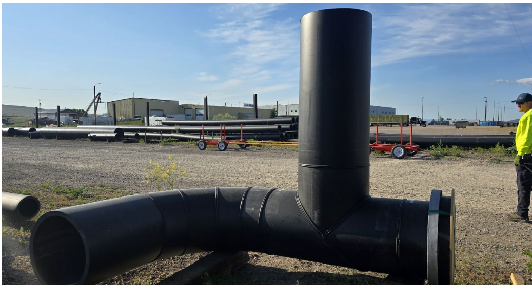
Image 1. Replacement HDPE tee in the fabricator's laydown yard.
