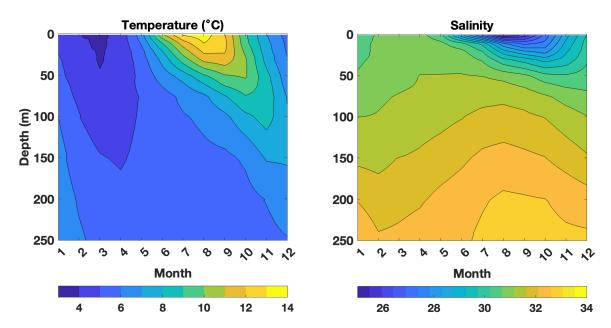
Figure 4. Monthly climatology of temperature (left) and salinity (right) from the best 53-year combined time series of the conductivity and temperature at depth profile and moored datalogger records.
