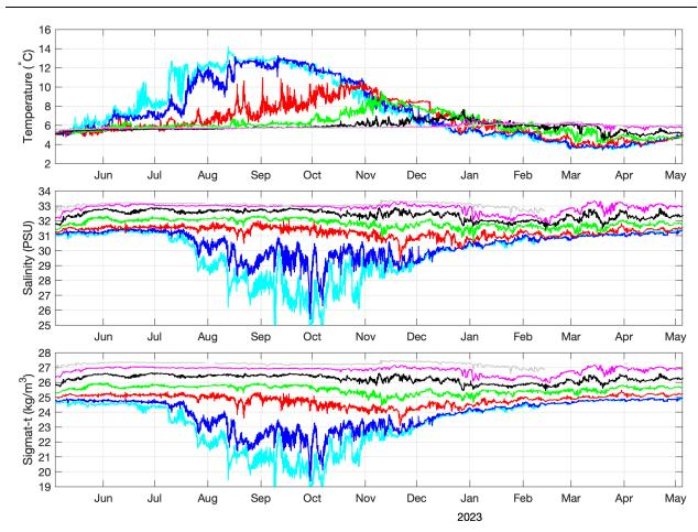
Figure 1. Data records from the 2021-2023 deployment of the GAK1 mooring, with temperature (top), salinity (middle), and density (bottom). Colors denote different instrument depths, with the 2023 sensors winding up near 19 m (cyan), 32 m (blue), 62 m (red), 102 m (green), 153 m (black), 204 m (magenta), and 254 m (gray).
