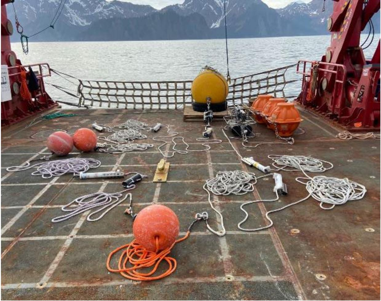
*Figure 5. The GAK-1 mooring assembled on the deck of R/V Sikuliaq prior to deployment in May 2020.*
