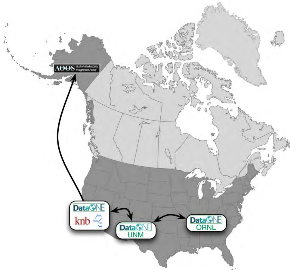
Figure D-3. Movement of data replicas in Member Nodes of the DataONE Network. The Gulf of Alaska Historical Data Metacat server is located in Santa Barbara, CA. Data are automatically replicated to the KNB repository in Santa Barbara, the University of New Mexico data repository, and the Oak Ridge National Laboratory repository. In addition, a copy of the historical data and metadata are manually copied to the AOS data system, headquartered in Anchorage.
