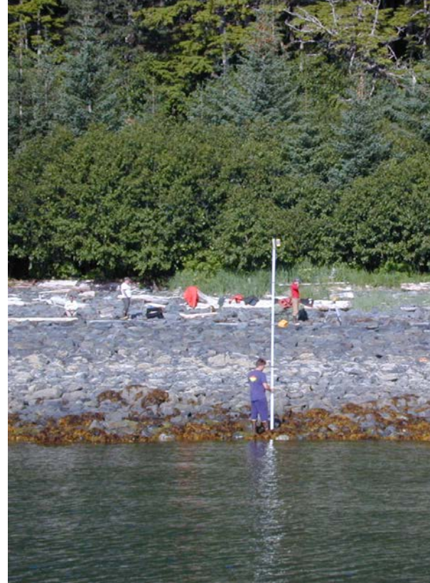
Finding Mean High Water Line using stadia rod and reciever.
