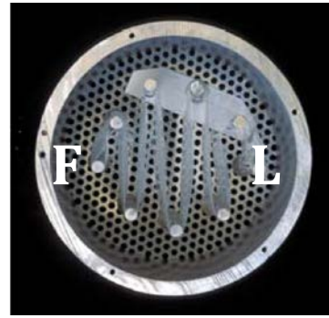
A successfully loaded puck: the first (F) and last (L) prongs are labeled.
