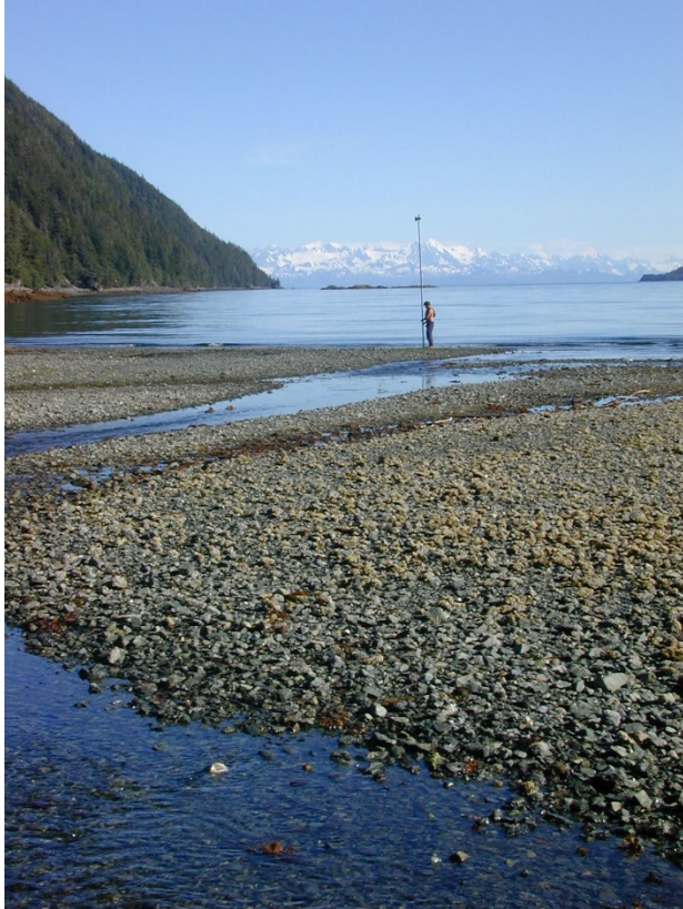
Finding Mean High Water Line using stadia rod and reciever.
