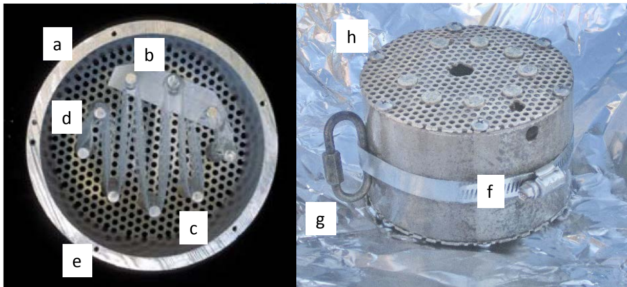
Anatomy of PEMD: a) aluminum housing, b) prongs affixed to wire mesh, c) wire mesh, d) LDPE strip looped on prong, e) holes for screws/mesh, f) hose clamps, g) D-ring or carabiner, h) stainless screws.
