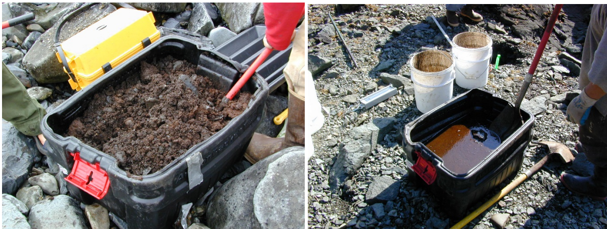
Tote with oiled pit contents being homogenized with a shovel.
