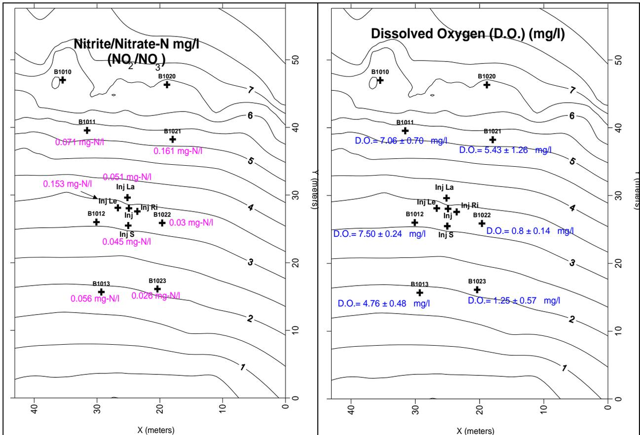
**Figure 8.** Plan view of beach EL056C, Northwest Bay, Eleanor Island. The landward direction is upward. The wells labeled B1010-1013 (Left) are in the unoiled transect; wells labeled B1020-1023 (Right) are in the oiled transect. Heavily oiled residue (HOR) was present at B1022 and B1023. The contours represent the topography in meters. The cluster in between the transects represents the injection well (in the middle) and the monitoring wells around it.
