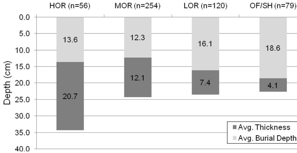
**Figure 1.** Average thickness of subsurface oiled layers and burial depth in cm below the surface by oiling descriptor based on data from pits in PWS surveyed in 2001, 2003, and 2007 (n=509). SO = surface oiling, SSO = subsurface oiling, OF = oil film, SH = sheen, LOR = lightly oiled residue, MOR = moderately oiled residue, and HOR = heavily oiled residue.
