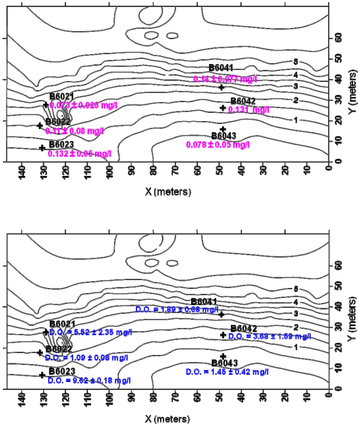
**Figure 9.** Plan view of beach SM006C, Smith Island. The landward direction is upward. Oil was present at well 6022. (Top) Average nitrate concentration (mg/L of N). Note that the optimal nitrate-N concentration for biodegradation of oil is 2 to 10 mg/L. (Bottom) Dissolved oxygen concentration at an average depth of 2.5 feet.
