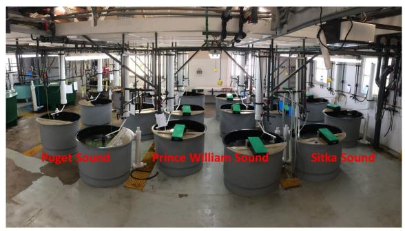
Figure 3. Footprint of the 18 grow-out tanks for oil-exposed herring, including duplicate tanks for unexposed, medium-low oil, and medium-high oil exposures for each stock (PWS, Sitka Sound, and Puget Sound).
