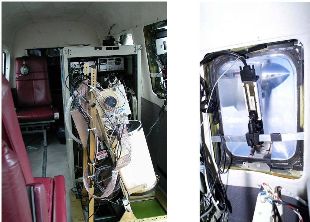
Figure 4. The photograph on the left is the NOAA-ETL fish lidar (telescope in the fore view with the hardware rack behind) mounted in the survey aircraft used in the summer of 2000. The photograph on the right shows the digital imager mounted in the window.
