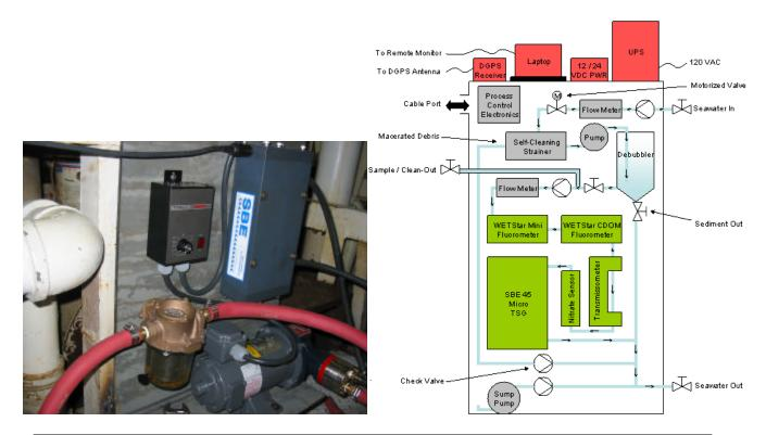
Figure 8. (a) A simple thermosalinograph installation with a sea strainer, pump and motor controller. (b) A schematic of a full flow-through sampling system with flow meters, automatic cut-off valves, self-cleaning sea strainer, debubbler, chlorophyll fluorometer, CDOM fluorometer, transmissometer, nitrate sensor and thermosalinograph.
