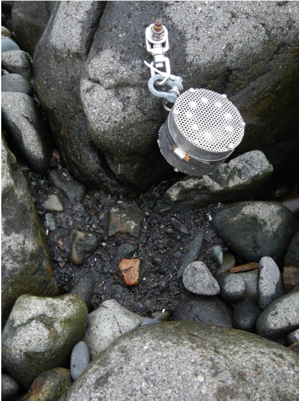
Figure 4. A passive sampler (PEMD) in a metal housing (11 cm diameter) bolted to a boulder at the Kiukpalik Island site in 2012. The sampler is deployed above a patch of remnant Exxon Valdez oil which has a surficial asphaltic layer covering little-weathered oil mousse. The passive sampler's purpose is to detect if oil constituents are being released into the water column.
