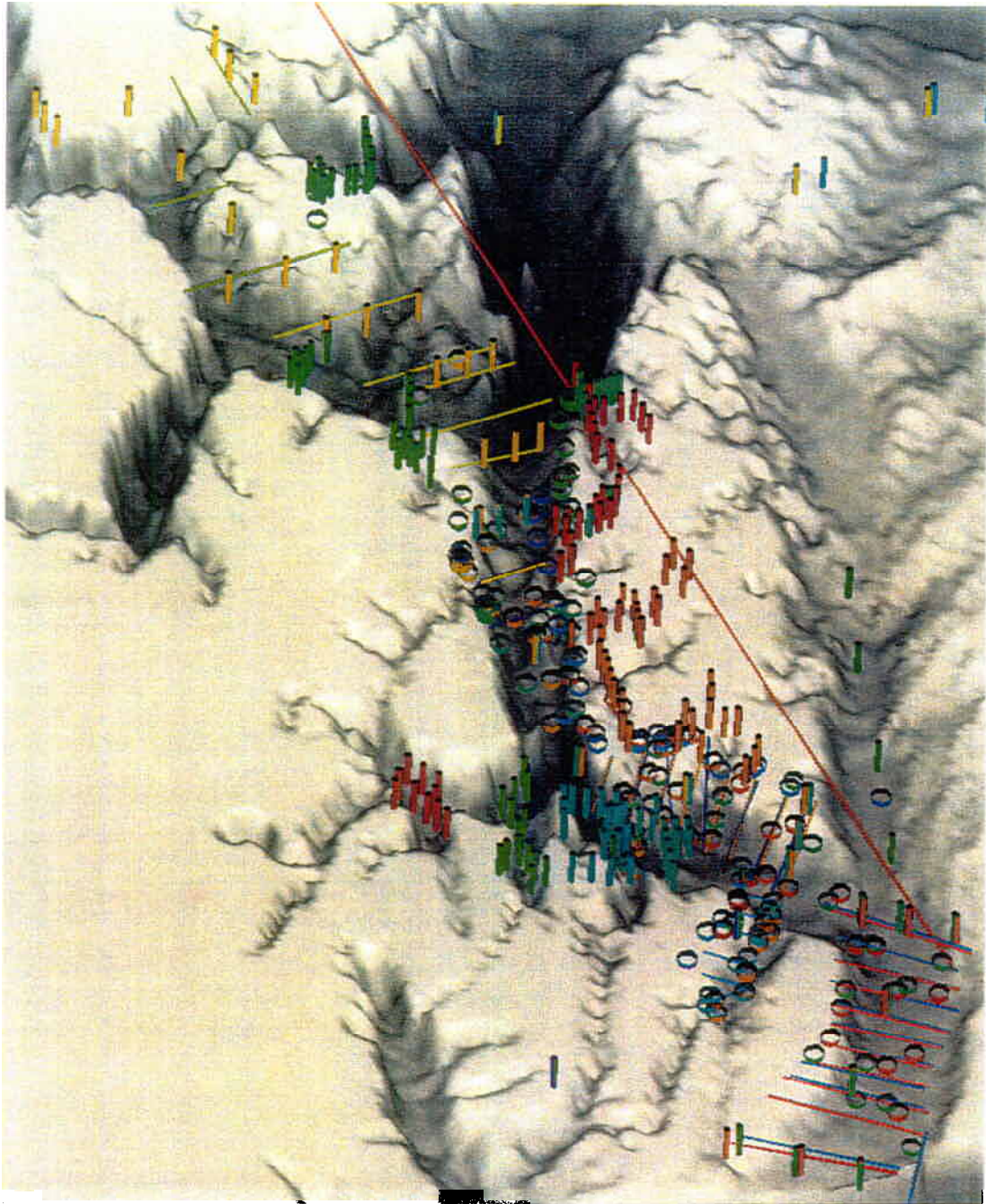
FIGURE 8: AVS image of the "western corridor" showing all sites sampled between June 15 and July 15, 1994, by CTD (vertical columns); hydroacoustics (horizontal lines), and midwater trawl (open circles).
