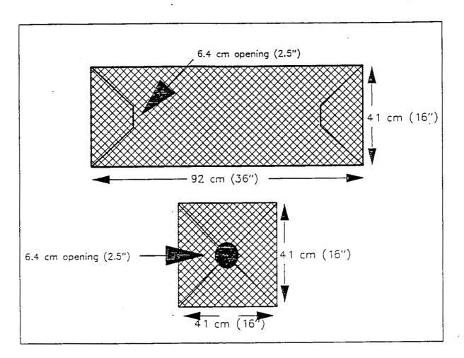
Figure 4. Specifications of the pots used to capture spot shrimp for the spot shrimp surveys.
