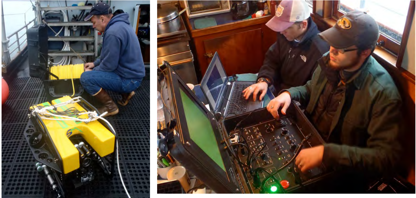
ROV and imaging sonar system (left panel) on deck and control system for the ROV and imaging sonar systems (right panel) during initial field testing.
