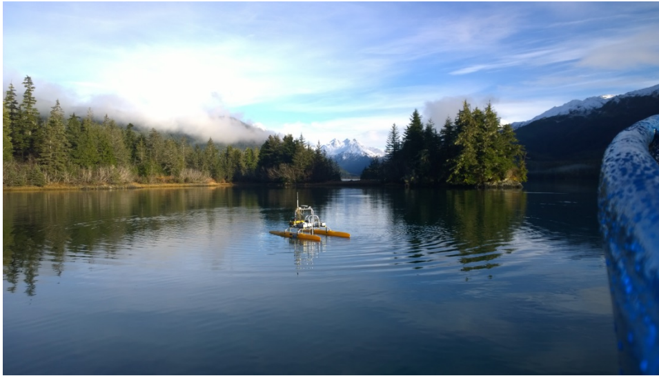
Figure 1. The autonomous surface vehicle (ASV) was deployed during our November 2015 cruise in all 8 bays to acoustically survey near shore waters to compare with observations in the main bay transects.
