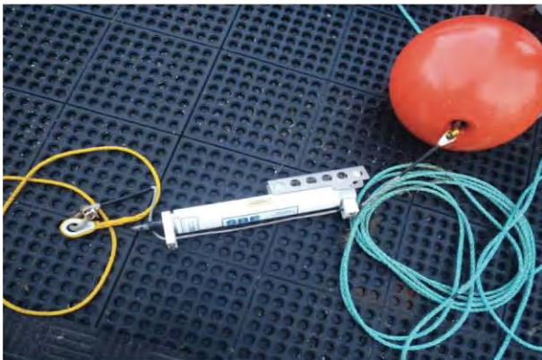
Fig. 2. Photos from the mooring cruise conducted in August 2010. a) near-surface CT (2m depth) showing fouling accumulated over the summer; b) vessel-mounted 150 kHz ADCP being calibrated during the cruise within Whale Bay; c) mooring preparation for re-deployment; SB37 microcat replacing the near-surface SB16 and placed at 5m depth.
