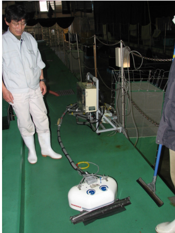
Figure 12. Photo of electric-eye sensing vacuum system used to clean tank waste.
