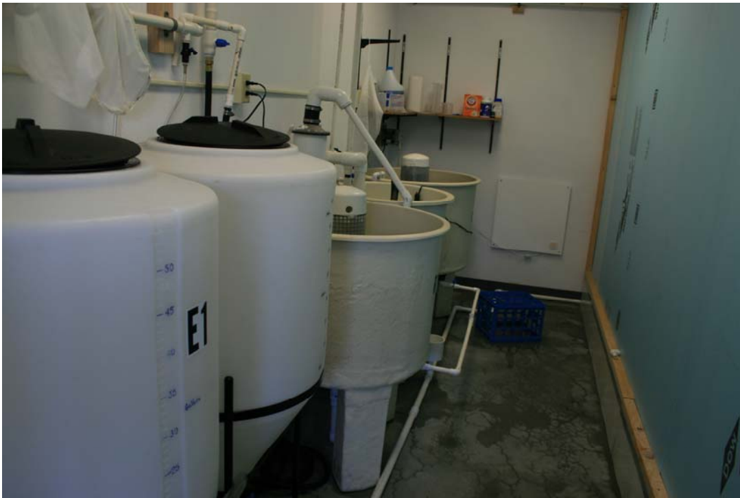
Figure 2. Larval herring culture tanks with degassing columns (a. top photo) and live feed culture tanks rotifers in rear and artemia in foreground (b. bottom photo).
