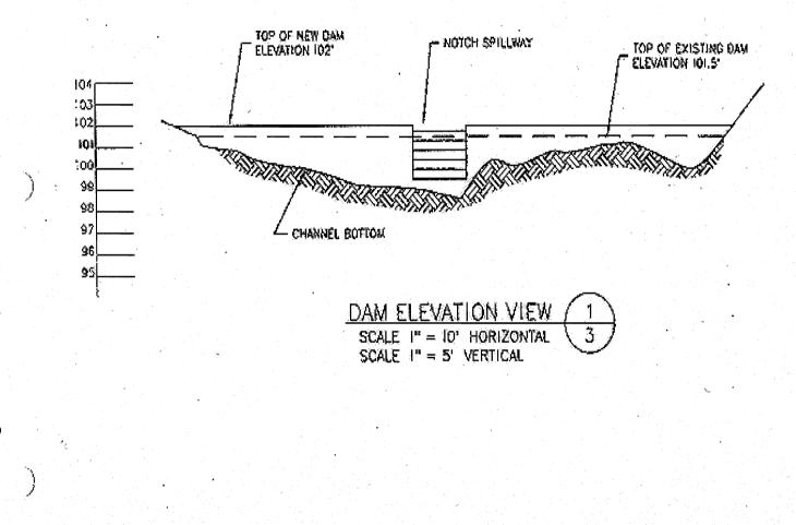
Appendix 5. Dam design at lake outlet (elevation view)
