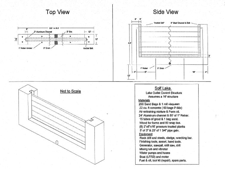
Appendix 3. Plan View of Installed Control Structure at Solf Lake.
