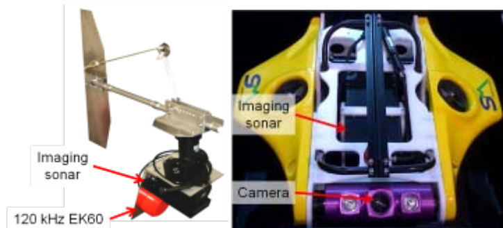
Figure 1. Deployment options for acquiring in situ estimates of fish length distribution. Left- Remotely controlled vane, comprising of two sonar systems, an imaging sonar (black) and traditional fisheries echosounder (orange) to be deployed at depth into herring schools for in situ size and density estimation. Right- ROV with fully articulating camera and imaging sonar, configured to share the same view, both can look forward and completely pan to -90 degrees, simultaneously viewing the same mass of water. The ROV was developed by Boswell and Seamor Marine specifically to integrate the imaging sonar into a towable body to track herring schools at depth in Lynn Canal.
