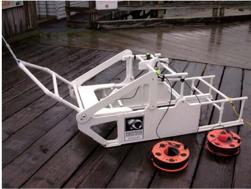
Figure 6.3. We constructed a video camera sled for monitoring the disposition of unprocessed fish waste at the experimental dump site and the relative abundance and distribution of scavengers feeding on the waste. The sled held two cameras that filmed the seabed as the sled was slowly pulled through the experimental dump site area.
