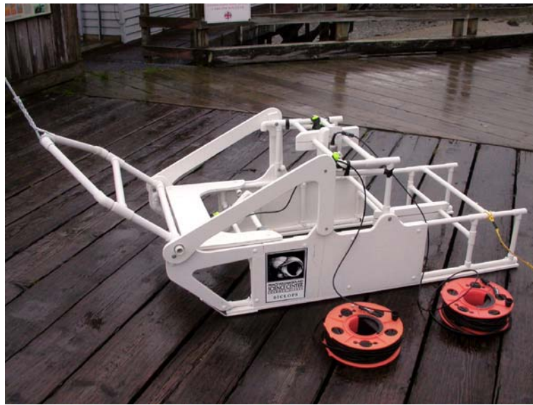
Figure 4. A special camera sled was constructed to monitor the distribution and decomposition of fish waste in the study area.
