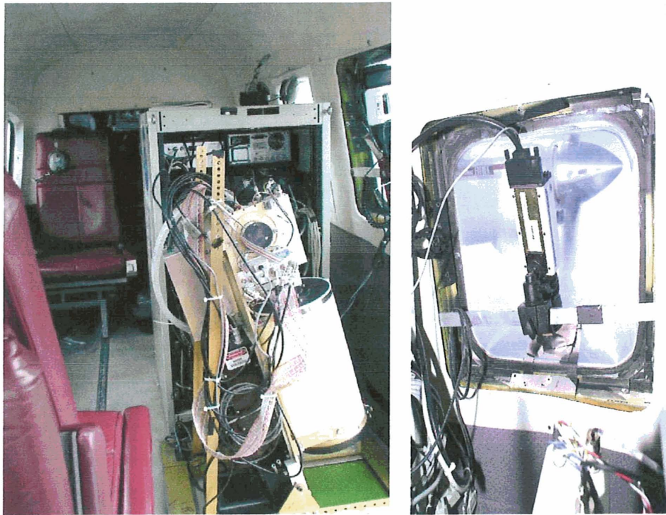
Figure 4. The photograph on the left is the NOAA-ETL fish lidar (telescope in the fore view with the hardware rack behind) mounted in the survey aircraft used in the summer of 2000. The photograph on the right shows the digital imager mounted in the window.
