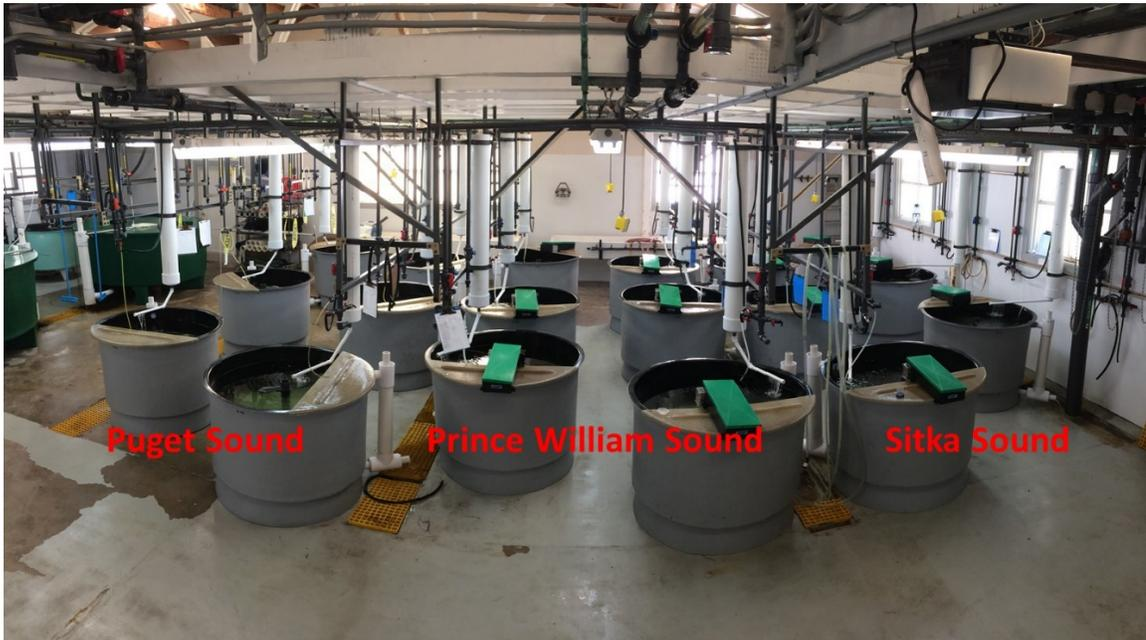
Figure 3. Footprint of the 18 grow-out tanks for oil-exposed herring, including duplicate tanks for unexposed, medium-low oil, and medium-high oil exposures for each stock (PWS, Sitka Sound, and Puget Sound).
