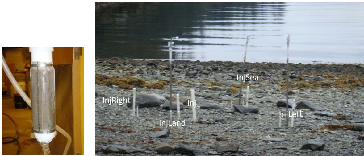
Figure 5: Left panel. The screen that covers the tip of the injection well (length of screen is approximately 0.30 m long, a foot). Right panel: Photograph of the HPI at Beach 1 (Figure 1). Copyright Groundwater Monitoring and Remediation, From Boufadel and Bobo (2011).
