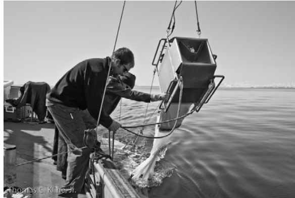
Figure 2.1. The Multinet being deployed horizontally in PWS. The codends of the five nets can be seen trailing in the water. The internal flowmeter is light in color and in the upper portion of the mouth. The external flowmeter and CTD hardware are on the outboard side of the Multinet so not visible here.
