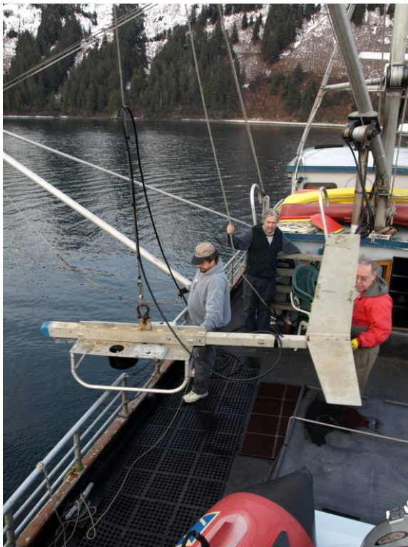
Fig. 27. Deploying the acoustic towed vehicle from the MV Auklet
