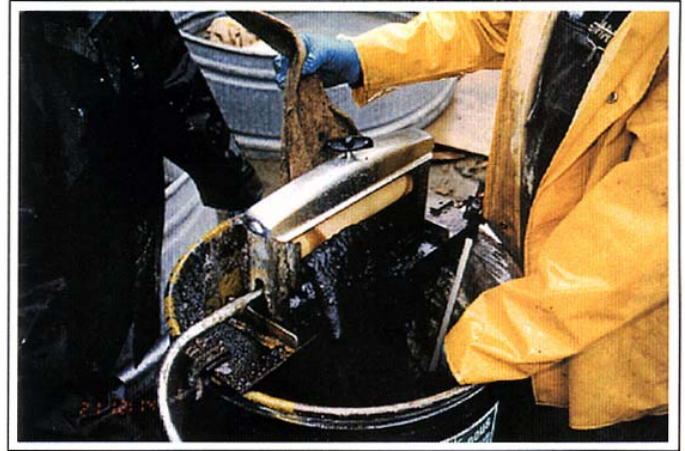
Extracting oil from sorbent pads to estimate oil content. Photo by J. Ginter
