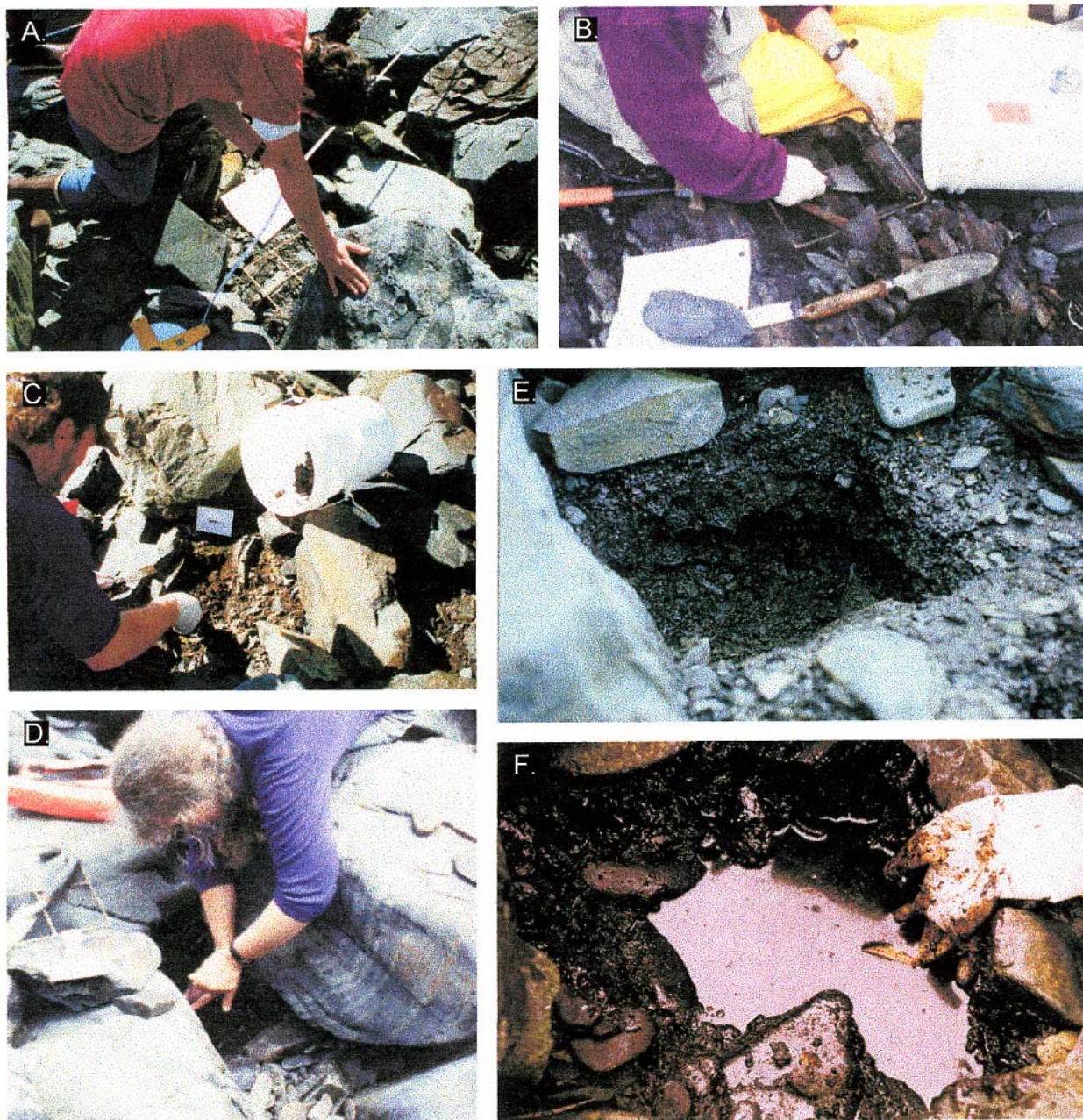
Figure 6-3 Methods used for oil sampling. A shows surveying of quadrant locations. B, C & D show excavating below quadrats. E shows a particularly dry sample hole. Note that oil is sticking the gravel together at the top few cm of the hole, allowing it to retain its square shape, but that unoiled gravel in the bottom of the hole has caved in. F shows a particularly wet and oily hole, with plastic glove for scale.
