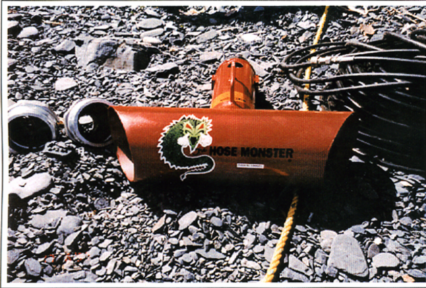
The Hose Monster®, an energy dissipater, was used to aid deluge flooding. Photo by D. Easton
