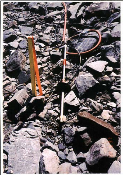
Modified airknife use for surfactant injection. Photo by D. Easton
