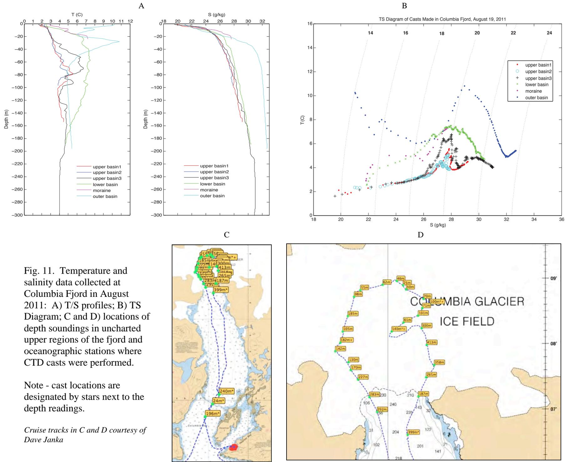
Fig. 11. Temperature and salinity data collected at Columbia Fjord in August 2011: A) T/S profiles; B) TS Diagram; C and D) locations of depth soundings in uncharted upper regions of the fjord and oceanographic stations where CTD casts were performed.
