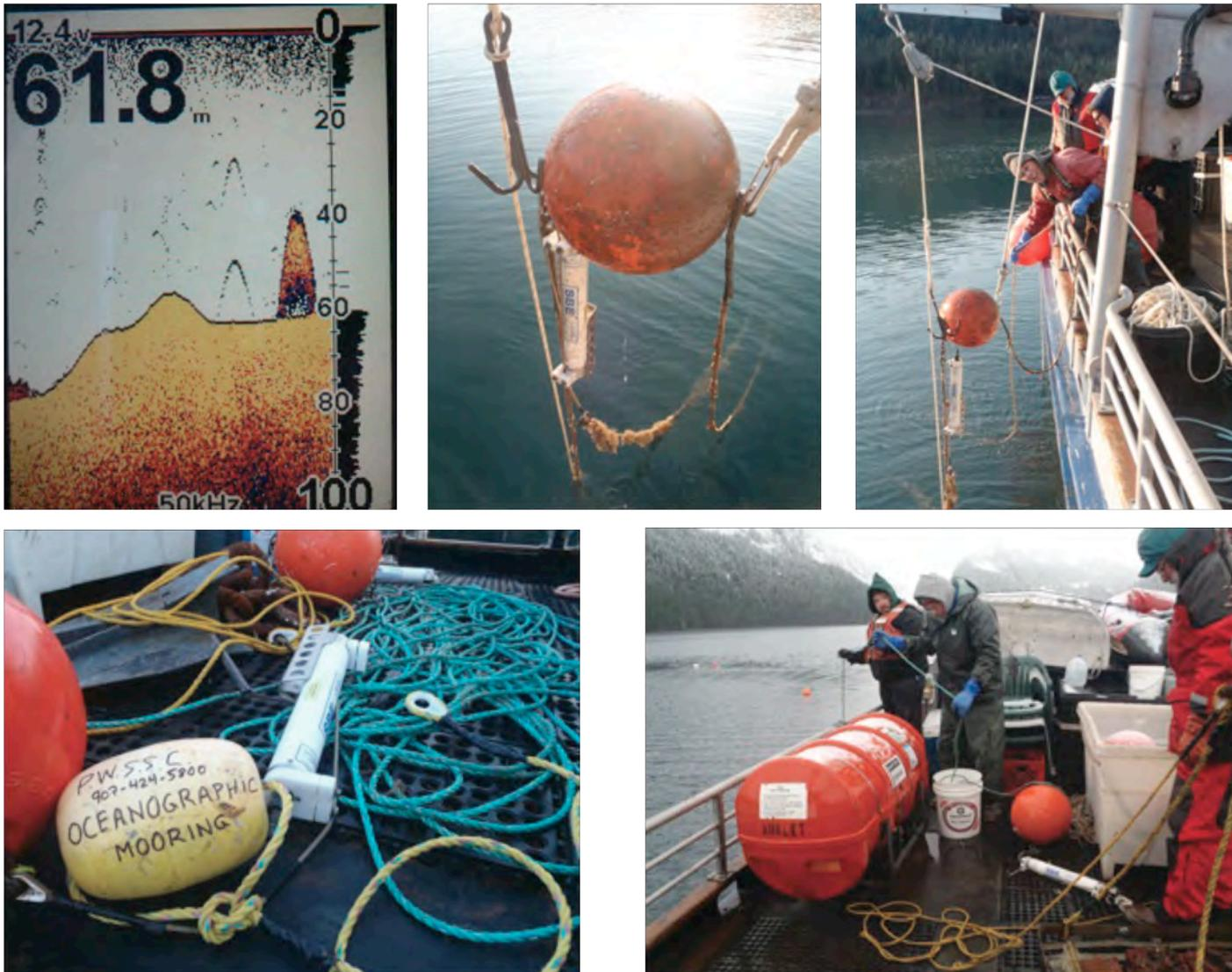
Fig. 2. Highlights from mooring cruise in April 2011. Clockwise from upper left: i) echo anomalies (large inverted V's) signifying the presence of submerged buoys and microcats; ii and iii) recoveries of moorings using garpplles following the loss of surface floats due to sheet ice; iv) mooring components in preparation for deployment at Whale Bay; and v) deployment of mooring at Eaglek Bay. (All above photos are courtesy of Dave Janka.)
