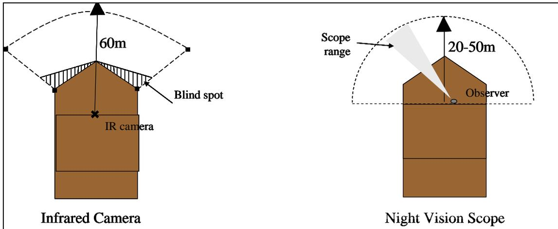
**Figure 1.** Comparison of survey fields for two night survey methods: (left) the infrared-mounted camera and (right) an observer equipped with a night vision scope.
