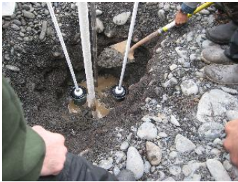
Figure 2: Placement of two Sampling Boxes, a multiport sampling well, and water level well (the white PVC pipe) in a pit.
