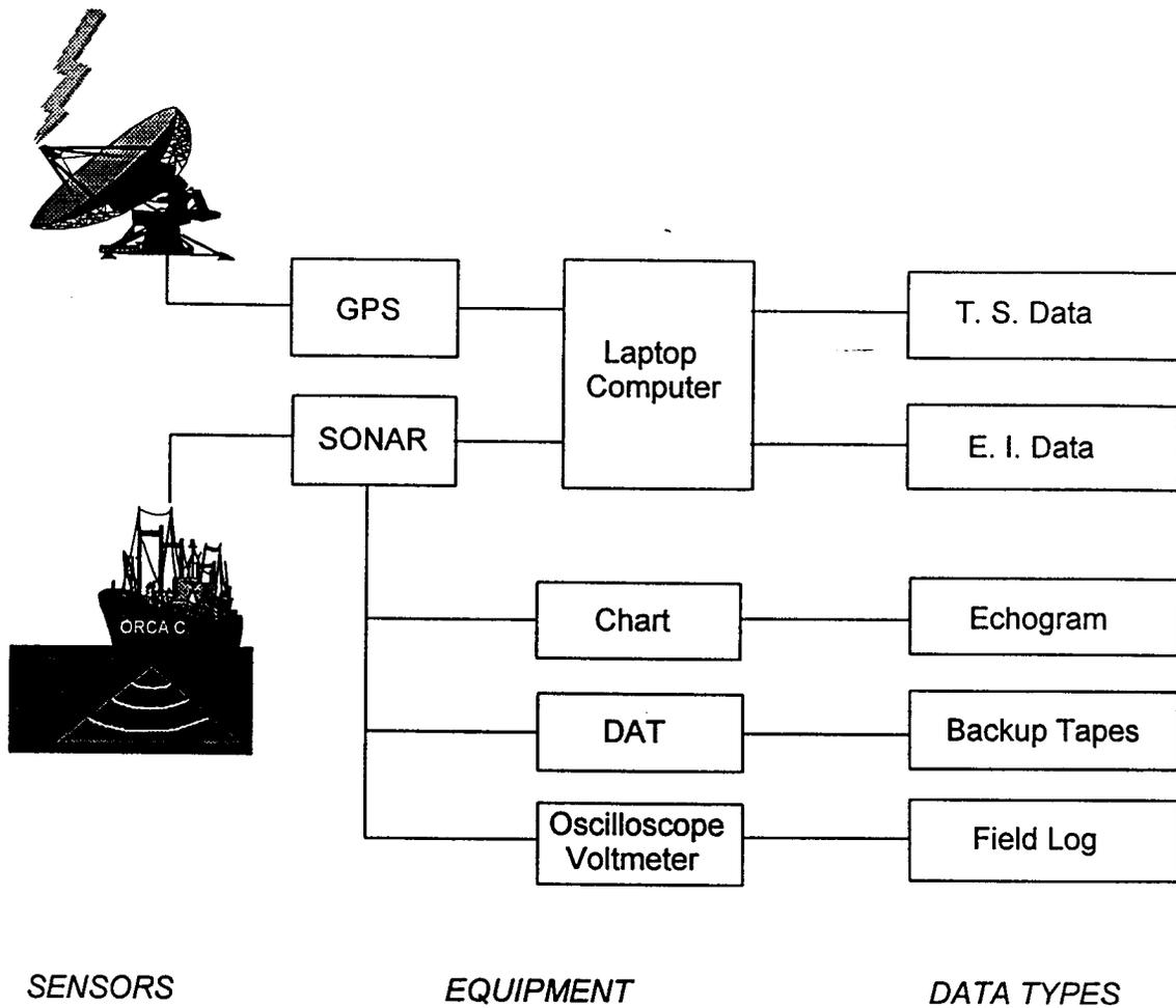
Figure 6. Data acquisition system used in SEA 1994 and 1995 acoustic surveys.
